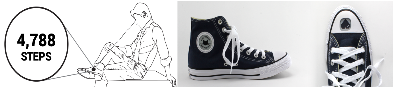
Figure 3: (Left) An example of the type of interaction afforded by a bistable e-ink display. (Right) The shoe prototype we designed and constructed. The e-ink display is embedded into the shoe [19].
