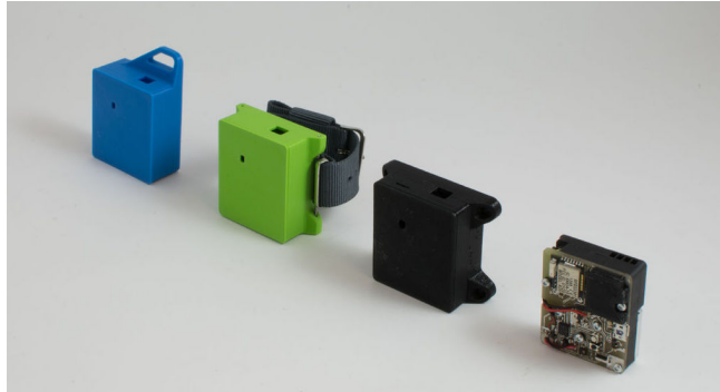
Figure 2: MyPart: a pocket-sized air quality sensor for personal, portable use in the outdoors with multiple form factors [18, 17].
