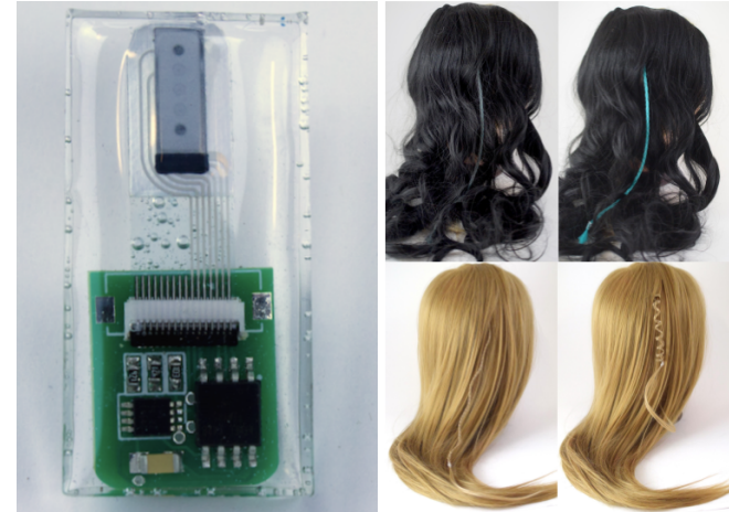
Figure 1: Left: Alternail circuit with microcontroller, e-ink display, and inductive coil for data and power transfer encased in resin. This fingernail-sized, battery-free interface is waterproof and hardy. Right: HairIO, an on-body system leveraging natural physical interactions for embodied interfaces [19, 5].
