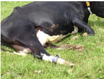
Figure 3: Wearable “anklet” on the leg of a dairy cow that uses accelerometers to track standing and lying behaviour in order to detect potential lameness (photo credit: [13]).
